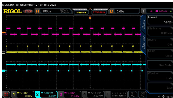
Figure 26. PWM rectifier IGBT SPWM pulses for three-phase
