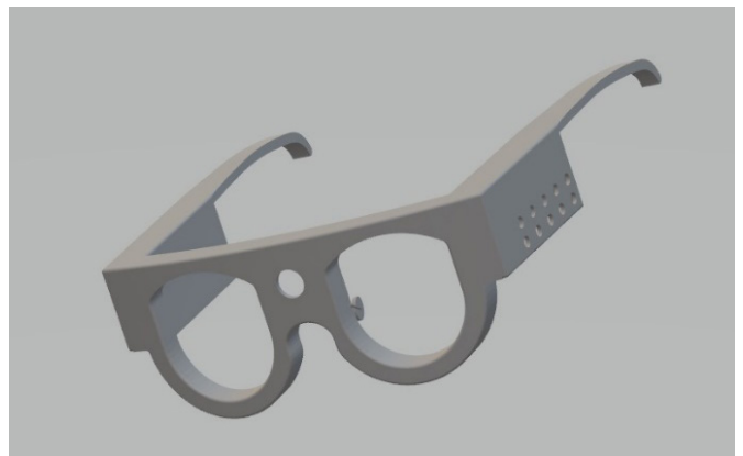
Figure 4. 3D CAD drawing of the glasses designed for partially visually impaired individuals
