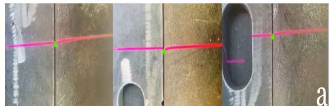
Figure 3. The test results of laser weld seam tracking for the butt joint
