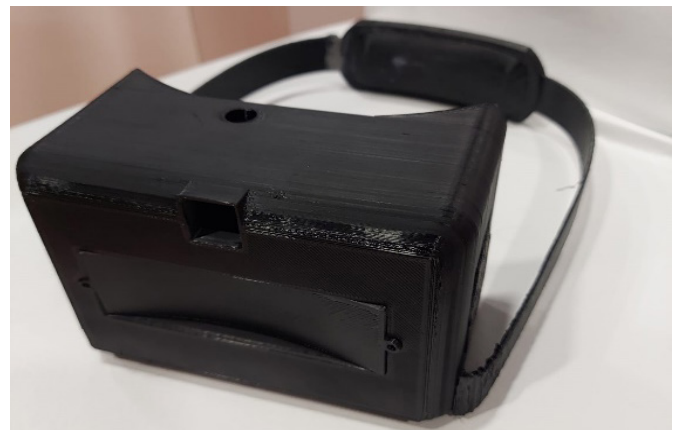
Figure 3. The prototype of the glasses designed for completely visually impaired individuals
