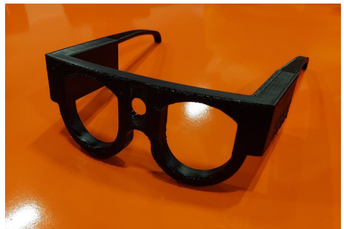
Figure 5. The prototype of the glasses designed for partially visually impaired individuals
